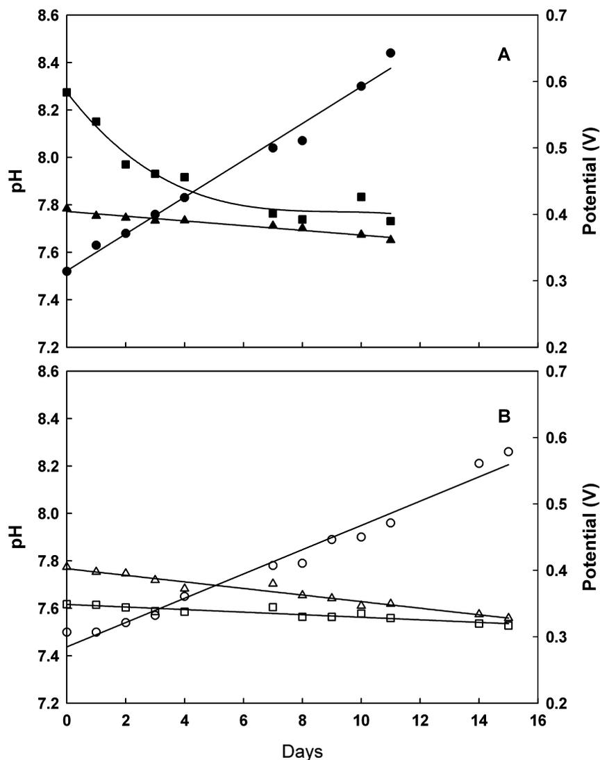
**FIGURE 3.** pH trends, cathode potentials, and overall cell potentials with nonreplenished phosphate-buffered catholyte: (A) AEM data for experiment C represented with solid symbols and (B) CEM data for experiment H represented with hollow symbols. Squares (■ AEM; □ CEM) indicate the overall potential across the fuel cell, triangles (▲ AEM; △ CEM) indicate the cathode potential, and circles (● AEM; ○, CEM) the catholyte pH.
