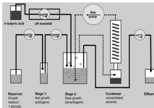
**Figure 1.** Schematic of two-stage continuous culture with gas stripping. The growth medium contained 60 g/L glucose as a source of carbon (for cell growth), and as a source of ATP and electrons for conversion of *n*-butyrate into *n*-butanol.
