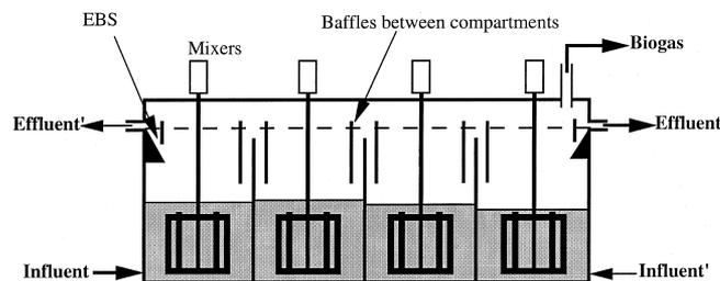
**Figure 1—Schematic diagram of AMBR (EBS = effluent baffle system).**
