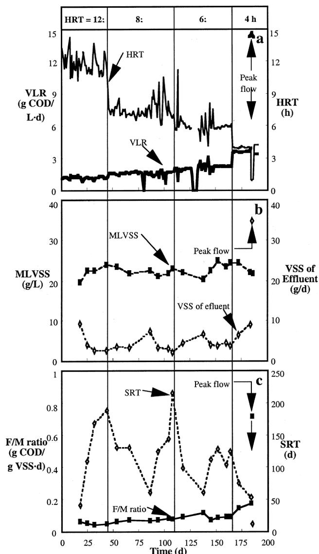
**Figure 2—Operating conditions: (a) loading conditions, (b) biomass concentrations in reactor and effluent, and (c) SRT and F:M. Results during the hydraulic stress test are indicated by peak flow.**
