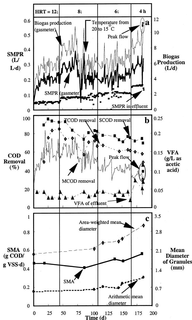
**Figure 3—Reactor performance: (a) biogas and methane production, (b) COD removal efficiency, and (c) biomass activity and granular size. Results during the hydraulic stress test are indicated by peak flow.**
