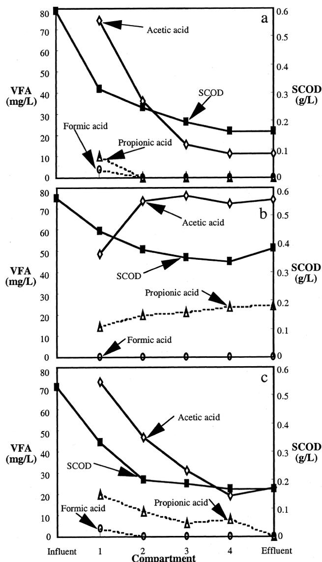
**Figure 5—Volatile fatty acid and SCOD concentration at the midpoint between intervals of flow per compartment: (a)  $t = 184$  days and general operating conditions at a 4-hour HRT; (b)  $t = 185$  days and hydraulic stress at a 1-hour HRT; and (c)  $t = 186$  days and day after hydraulic stress at a 4-hour HRT.**
